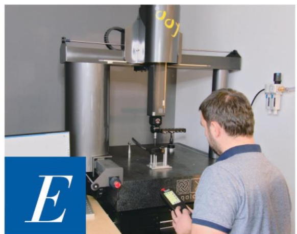
Machine for geometrical measurements (Aberlink Axiom too HS)
