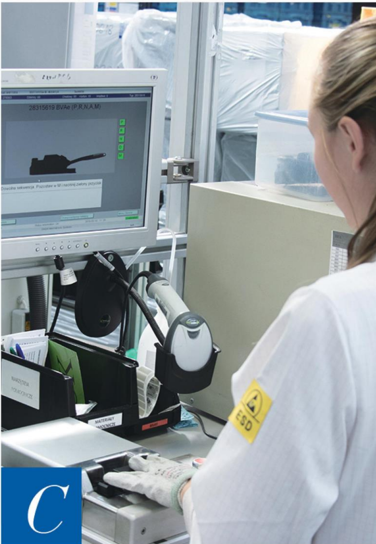
End of line tester (100% products tested)
