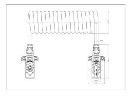
7P/12V Spiral Cable (Auxiliary, yellow) Conductors: 4x12ga + 2x10ga + 1x8ga
